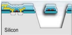
This technology is based on standard CMOS or BiCMOS process allowing integration of MEMS sensor and front-end electronic on the same die for better signal to noise ratio. Suspended passive devices or structures can be made with this technology. Applications include thermal inertial sensors and infrared sensors.
