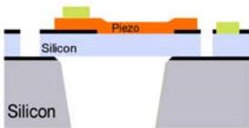
On-chip suspended membrane with piezoresistors
