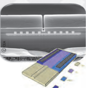
Lateral Ge PIN diode
