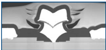
Thick gate metal results in low Fmin and low Rn, forgiving LNA matching
